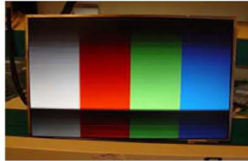
Horizontal Block Gate TAB IC Defect
